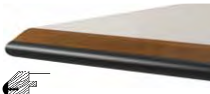
38177 1.25" x 1.25" beveled wood edge ½" vinyl T mold edge, black high pressure laminate, veneer, or Veneer Art top surface
