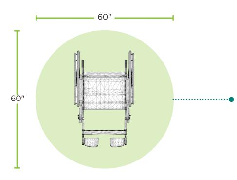
In order for a wheelchair to successfully manuever around a room, you must allow for 60" from the wall to the front of knee clearance
