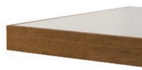
2300 / 2308 Wood Band 1-1/4" laminate top. The edges are banded with 1/4" hardwood. No radius at corners. Modesty edge Flat Wood Band
