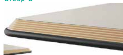
15177 1.25" 21-ply plywood edge .5" vinyl T mold bumper, black high pressure laminate top surface 3" standard radius corners
